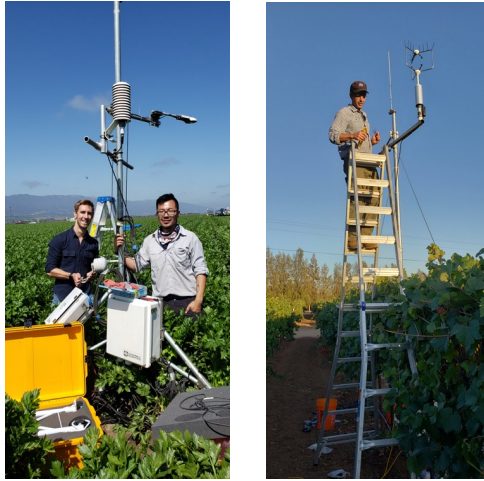
Deployment and maintenance of flux towers at validation sites for vineyards and celery.
